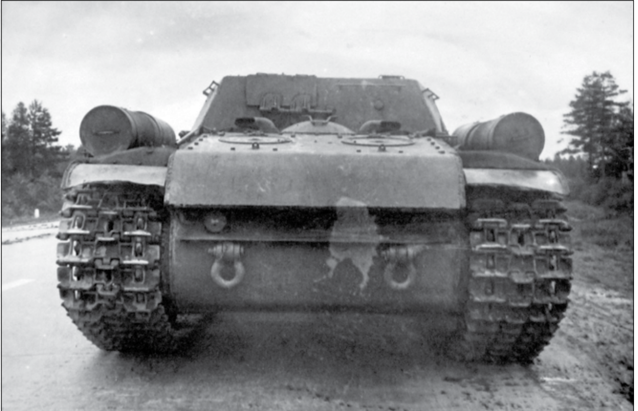
Rear view of the SU-152 produced between March and July 1943. The hand grab design had been simplified, and the edges of the superstructure and rear hatch were more roughly finished (TsAMO).
