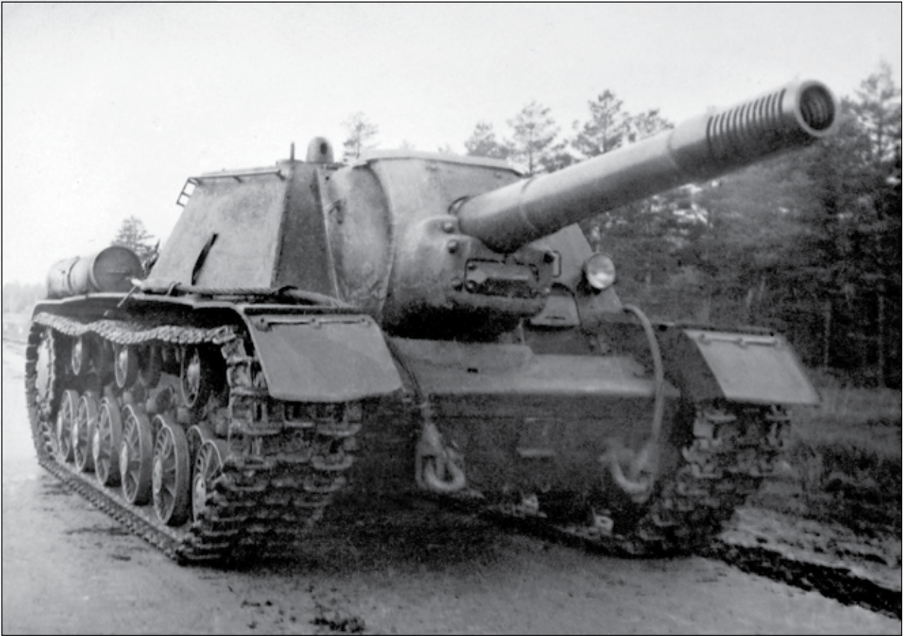
An SU-152 produced between March and June 1943. A pickaxe is visible on the right side; the attachment for it appeared in March 1943 (TsAMO).
