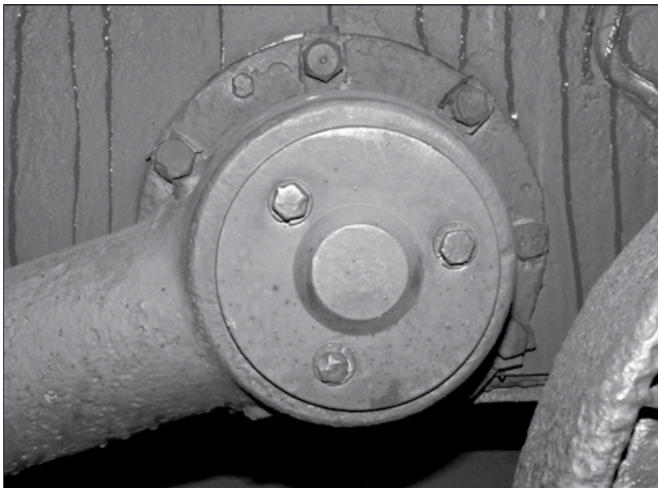
One type of bogie bracket cap used on SU-152's during the spring and summer of 1943 (YuP).
