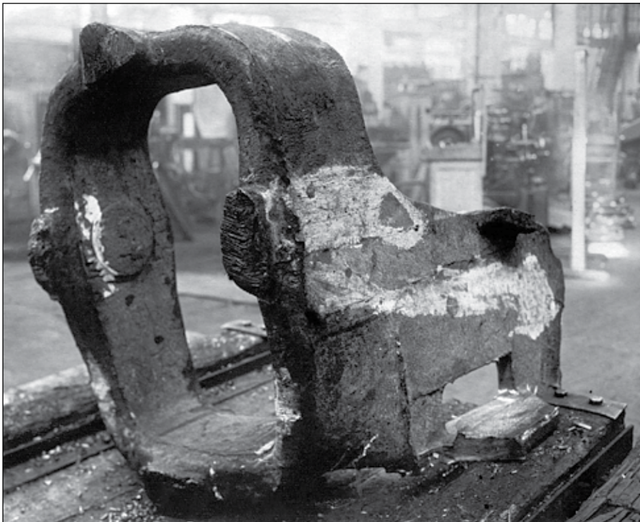
Experimental Bessemer steel frame for the ML-20S system manufactured at Factory No. 40 in March 1943 (TsAMO).
