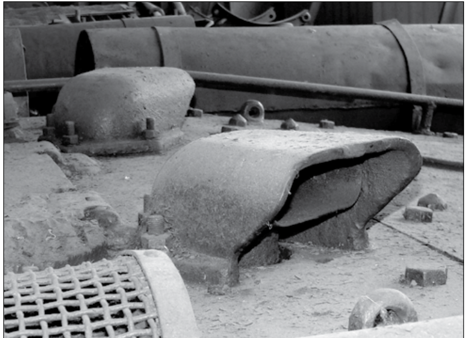
Modified exhaust stack shield introduced for the SU-152 and the KV-1S in late July 1943 (YuP).
